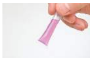
A high level of nitrite (formed from ammonium and is harmful) is shown (0.5mg/L)
